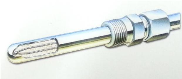
Thermocouple are pairs of dissimilar metal wires joined at least at one end, which generate a net thermoelectric voltage between the open pair according to the size of the temperature difference between the ends, the relative Seebeck coefficient of the wire pair and the uniformity.
